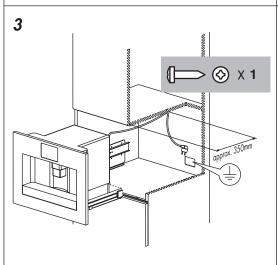
Fix the power cord with the special clip, to avoid the cord entangling when extracting or inserting the appliance.
