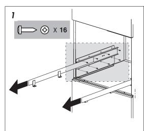
Lean the runners to the surface of the furniture. Fix the runners with the screws provided; then completely extract the two runners.
