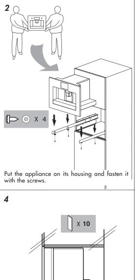
To align correctly the appliance, put the spacers under the bar's support.
