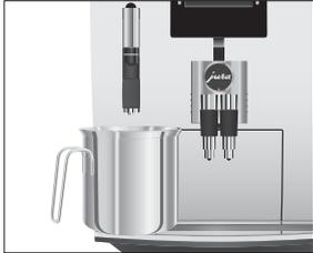
In order to protect the JURA from frost during transport, the system must be emptied.
