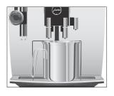
'System is filling', water flows out of the cappuccino frother. 'Empty drip tray'
